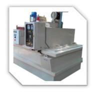
MEG has also installed an HCI Neutralization and Flux Regeneration Plant. These units are capable of regenerating more 90% of spent chemicals, which reduces the wastage and increases the economic value alongside reducing the environmental damage.
